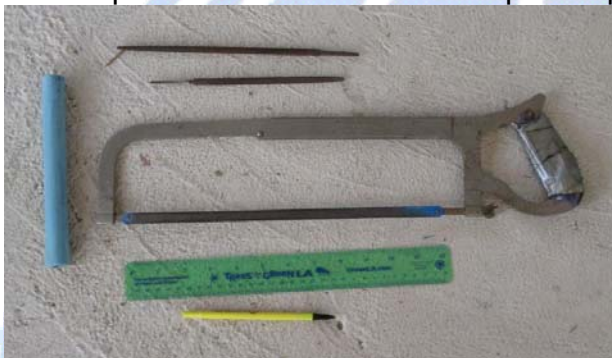
Phase 1 Tools for cutting the scrap PVC
