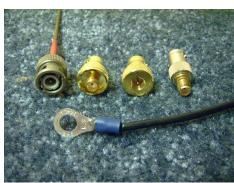
Some of the HT's sold today have different type male/female SMA connectors all SMA-to-BNC adapters pictured were bought from eBay. HT's are most difficult to quantifiably measure antenna performance from - you will just have to do it the old fashion way of over the air reports flipping between using a ducky vs. Whip+Tail under the same conditions, to judge.
