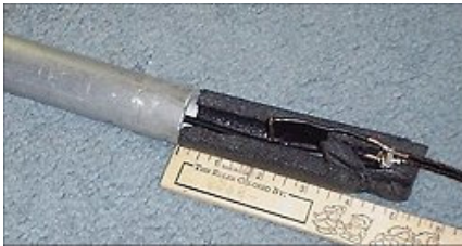
Picture B. Feed Point.
